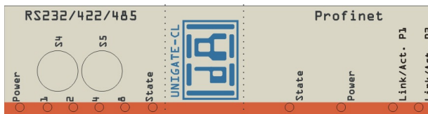
Picture 2: Front panel: Rotary switches and LEDs
